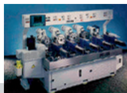
Chipless shaping and finishing by rotary swaging technology
