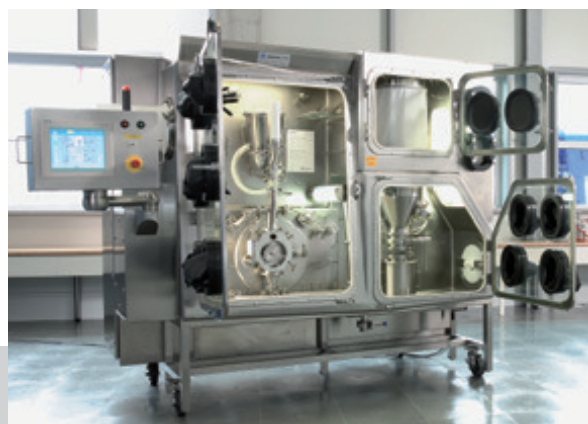
Isolator with integrated powder processing system
