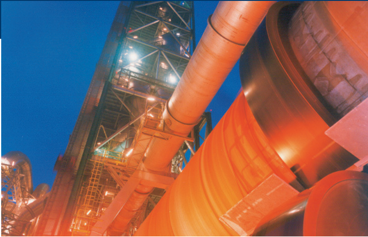
Pre-heating tower with rotary kiln of a cement factory
