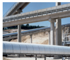
Curve-capable belt conveyors
