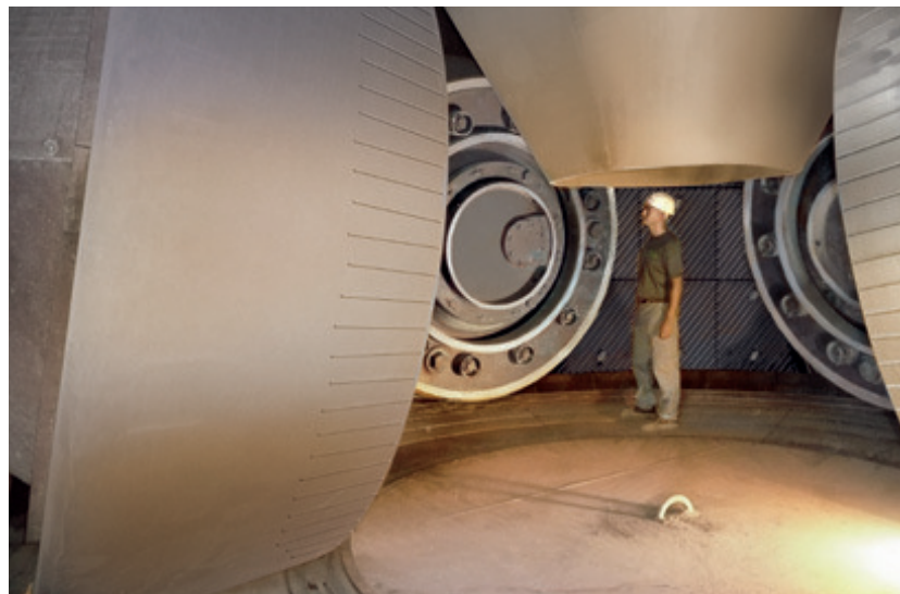
Interior view of a LOESCHE mill, type LM 60.4, with 4 rollers
