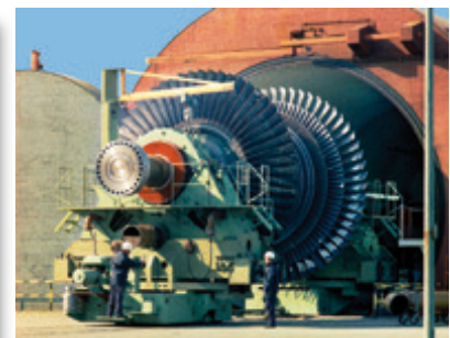
Rotor of a low pressure turbine in front of the balancing bunker
