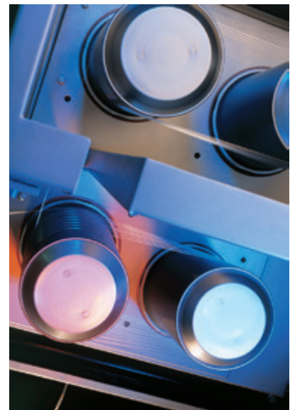
Heated draw roller modules for prestretching filament yarn
