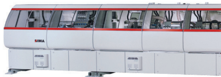
Edge treatment machine, type Novimat, including the KFA contour milling aggregate incorporating the latest linear technology
