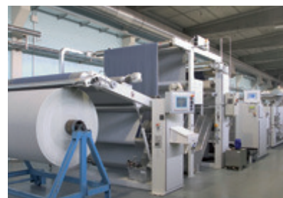
BRÜCKNER POWER-LINE tension machine: Exit – batch winder with peripheral drive, changeover roller and interim product storage trough
