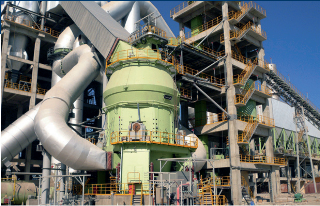
LOESCHE mill, type LM 60.4, for grinding raw materials
