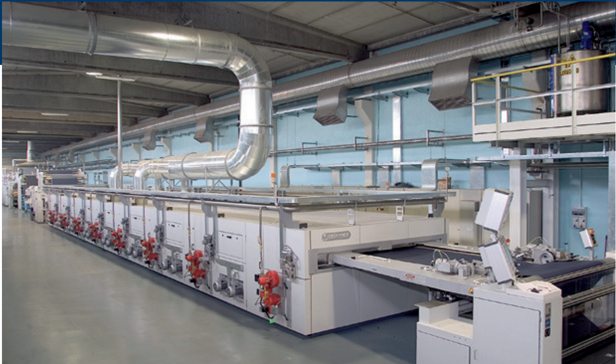
BRÜCKNER POWER-FRAME tension machine with patented "split-flow" ventilation system.
